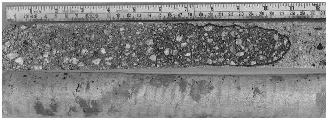
Fig. 9. Flow profiles (upper) and pipe wall surface (lower) Mix 3 – rubber, v = 0.2 m/s.
