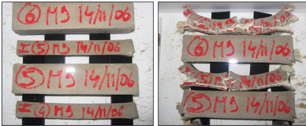
Fig. 4. M9 mortar specimens after 105 and 150 days in 30 g/L sulphate solution.
