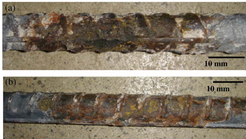
Fig. 5. The distribution of corrosion products on the rebar surface at a mid-section crack in (a) OPCC and (b) HPC.
