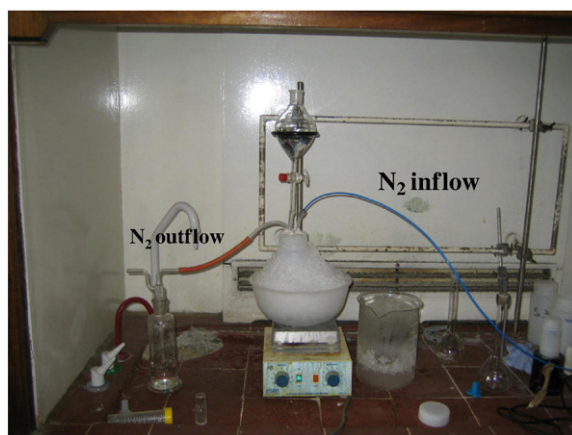
Fig. 1. Photograph of the apparatus used to synthesize C-S-H gels.
