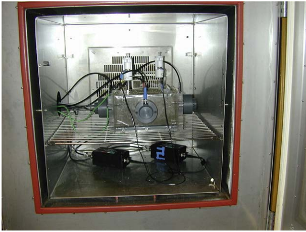
Fig. 2. The sample is placed in a climate chamber, closed without active control, diminishing outside temperature and relative humidity fluctuations.
