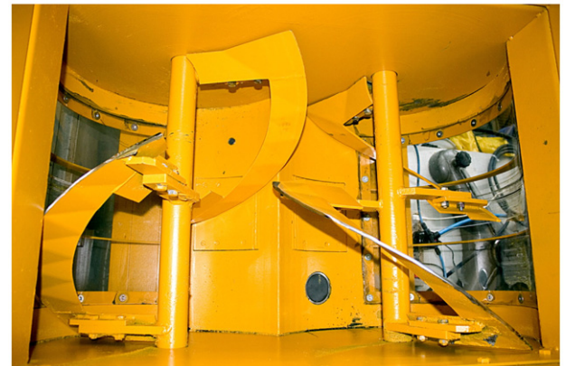
Fig. 5. View of mixing of ELBA-Laboratory single-shaft chamber ELBA and Laboratory mixer twin-shaft mixer.
