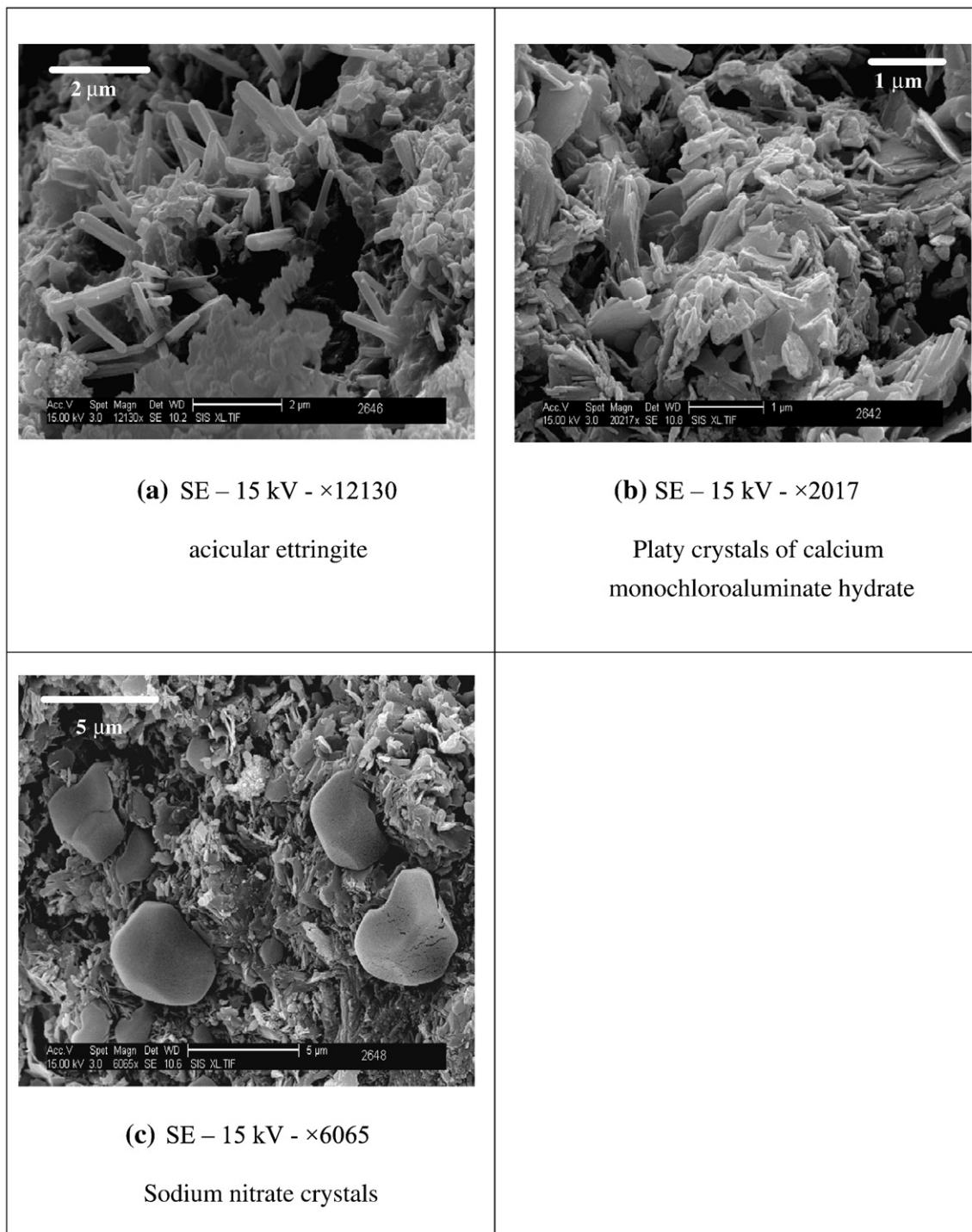
Fig. 6. SEM observation of a sample prepared according to formulation III (see Table 6) and cured for 6 months in sealed bag at room temperature.
