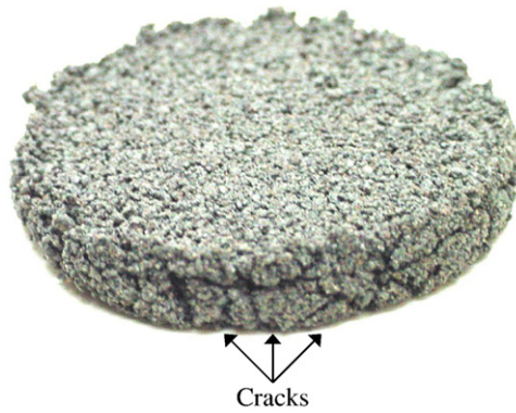
Fig. 4. Picture of the 13%-water sample tested 60 min after mixing with a displacement rate of 0.01 mm/s. Final height = 7.5 mm.
