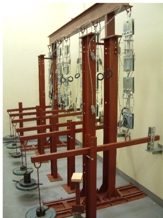
Fig. 1. a) The dimensions of the tensile specimens for the creep tests. b) The tensile creep frame.
