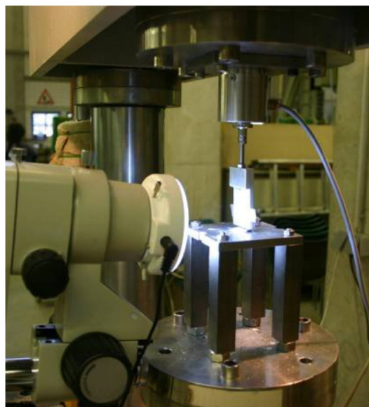
Fig. 4. The single fibre pull-out test setup.
