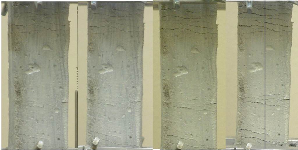
Fig. 13. Photos taken of one of the pre-cracked tensile creep specimens loaded at 80% of the tensile strength. The time after loading is from left to right: 30 min, 12 h, 6 days and 8 months.
