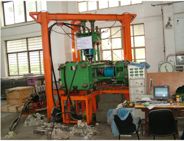
Fig. 2. The triaxial testing machine.
