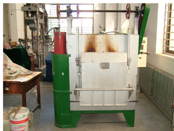
Fig. 1. The box-type electric furnace.
