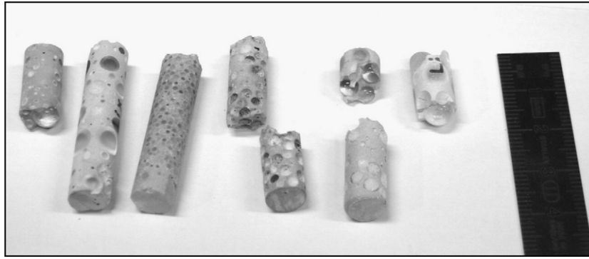
Fig. 2. Different cementitious composite specimens ( \phi 8 mm) after various degradation processes (leaching, drying and thermal exposure).
