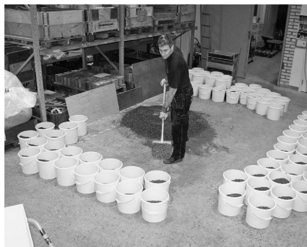
Fig. 19. Fractional shovelling, in accordance with EN 932-2.
