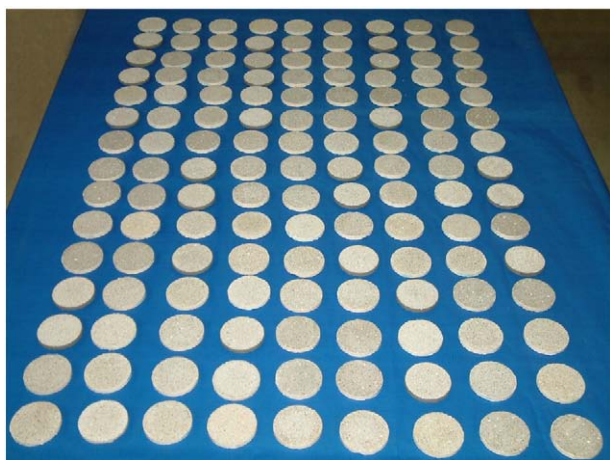
Fig. 1. Photo of the cement mortar samples used in the experiments.
