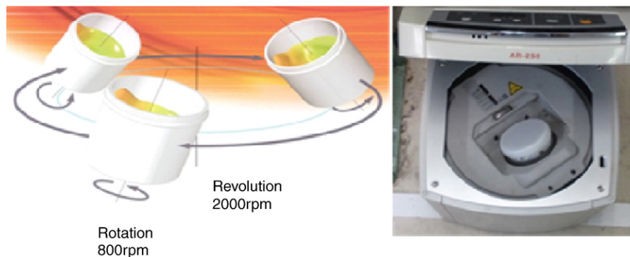
Fig. 1. Revolution/rotation propeller-less blending system deforming conditioning mixer (Thinky Corp. model AR-250).
