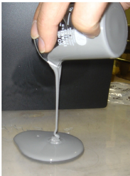
Fig. 2. Fluidity of calcium aluminate based DSP paste ( W/P=0.1 ).
