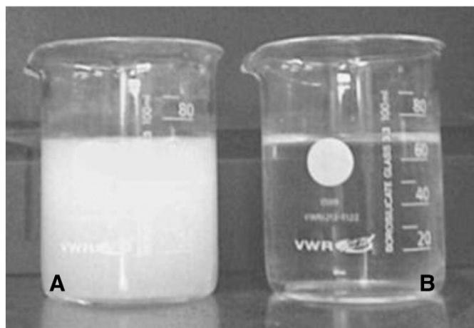
Fig. 5. \text{Ca}(\text{OH})_2 saturated solution precipitation test. A: GC. B: control.
