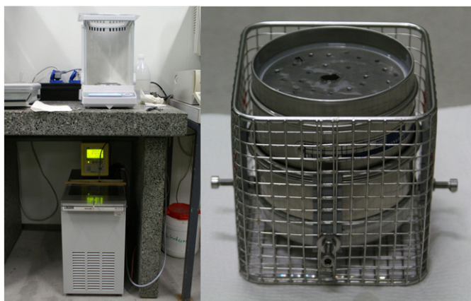
Fig. 2. Left: test setup with balance and thermostat. Right: permeable box, complete with upper removable and lower fixed sieve with holes for rapid circulation of the buoyancy liquid and permeable basket for fixation of the sieves.
