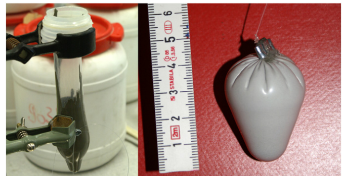
Fig. 1. Left: condom filled with cement paste fixed to a plastic ring, clamp and string during the filling procedure. Right: sample of cement paste ready for measurement.
