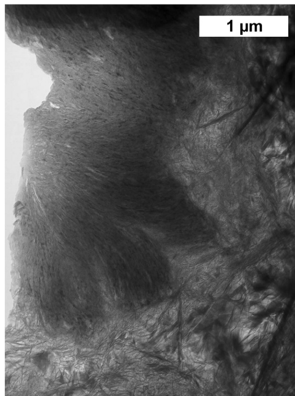
Fig. 16. A TEM micrograph from the KOH-activated paste hydrated for 28 days showing microcrystalline CH intermixed with C–S–H (left) and foil-like Op C–S–H (right and bottom).
