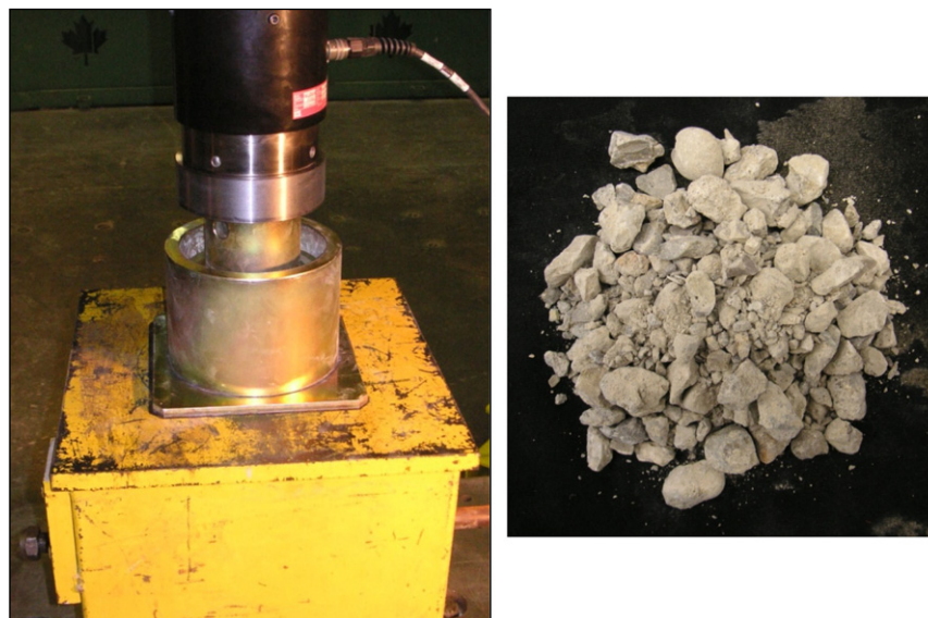
Fig. 2. Aggregate crushing value test setup and crushed RCA-1.
