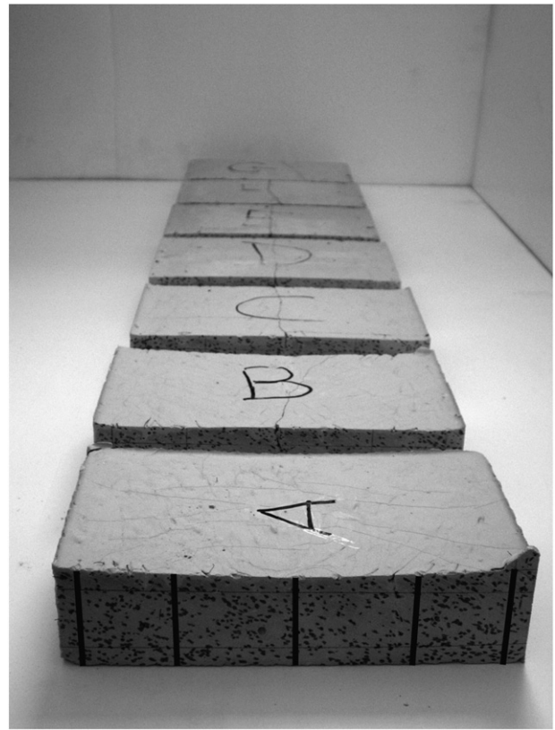
Fig. 10. Tested cut samples from the element after casting and studied sections. Fiber counting is performed on each of the six areas shown on the section.
