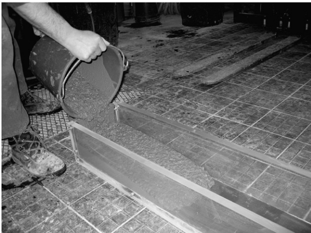
Fig. 9. Casting process in the channel formwork.
