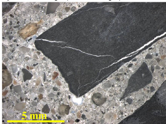
Fig. 3. Polished section of investigated concrete sample. a) ASR damage (crack with gel). b) Mechanical damage (empty crack).
