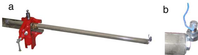
Fig. 1. a) Experimental set-up in the measuring position for the EMM-ARM; b) accelerometer detail.
