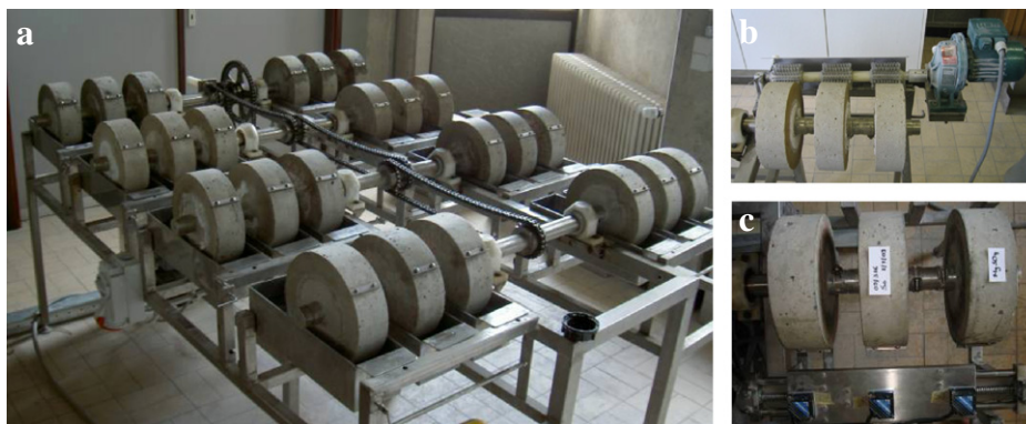
Fig. 1. Apparatus for accelerated degradation testing of concrete specimens.
