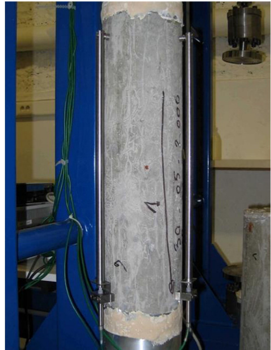
Fig. 15. Photo of the longitudinal displacement system.
