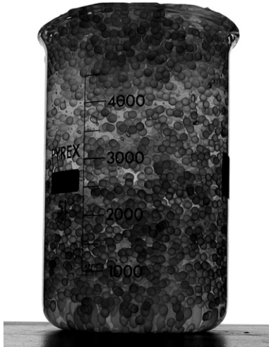
Fig. 3. Homogeneous carboxypol gel and glass beads mixture at the end of the mixing phase.
