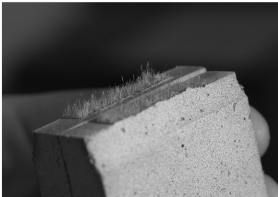
Fig. 18. Single crack obtained with specimen used for the image analysis of cracking.
