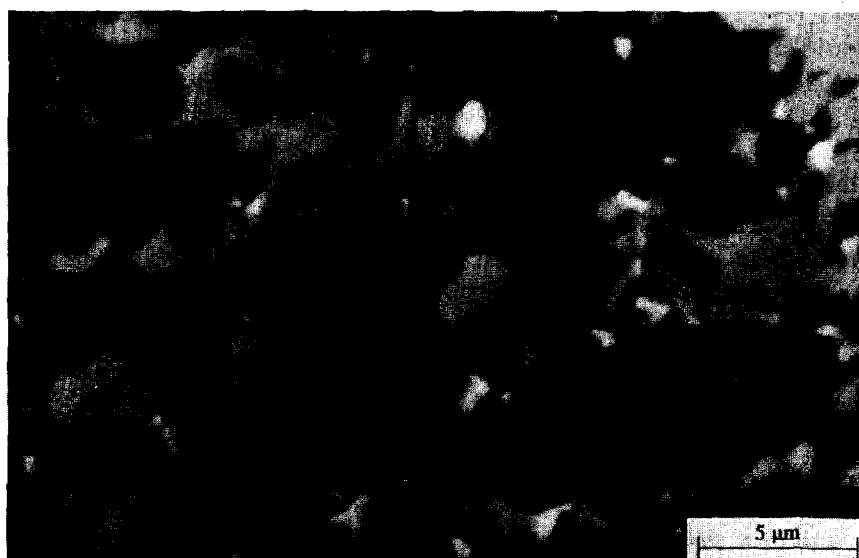
Fig. 2. SEM photograph of polished surface of the \text{TiB}_2\text{-Ti}_{0.5}\text{N}_{0.5} composite, heavy grey phase is \text{TiB}_2 , light grey phase is \text{Ti}_{0.5}\text{N}_{0.5} , bright phase is Ni and the dark region is pores.
