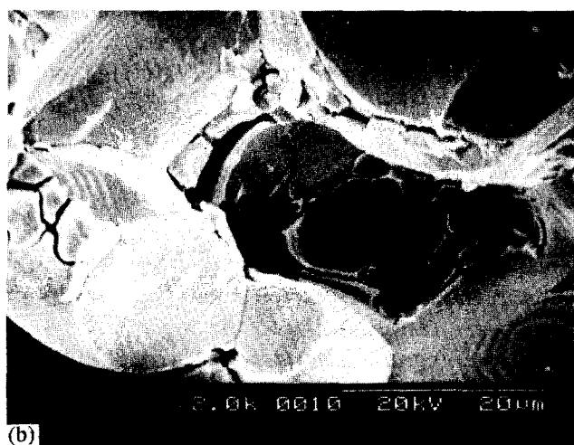
Fig. 7. SEM micrographs of the transition alumina coating in the \alpha \text{Al}_2\text{O}_3 filter: (a) example of layer obtained by sol-gel impregnation technique; (b) pore plugging after three impregnations with precursor C.
