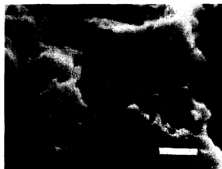
Fig. 5. SEM micrographs of unseeded composite 3.1- \text{A}_0 gel heated at 1400°C (bar = 1 \mu\text{m} ).
