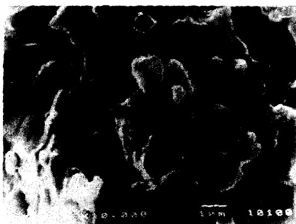
Fig. 7. SEM micrograph of N_8C_6 pigment, small size prismatic crystals in aggregate.
