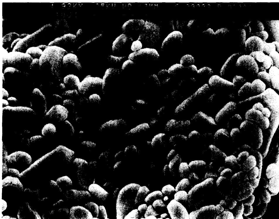
Fig. 6. SEM of fracture surface of 5% seeded boehmite with 0.5% niobia and sintered at 1400°C for 100 min.
