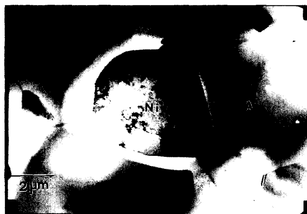
Fig. 10. Typical microstructure observed for the \text{Al}_2\text{O}_3/\text{Ni} composites. The microcrack is arrowed. A stands for alumina.
