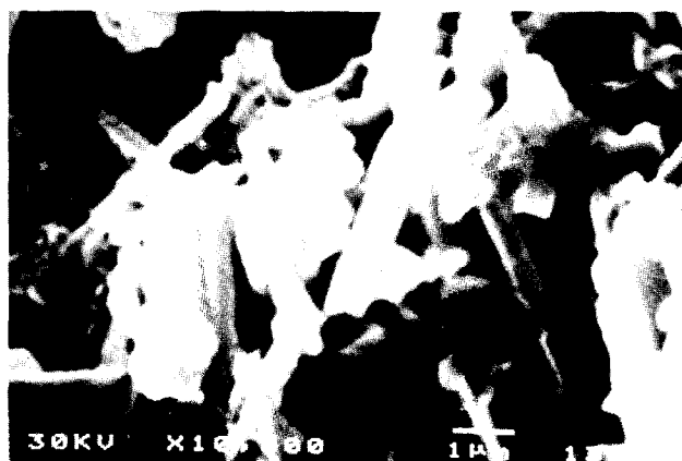
Fig. 6. Prismatic well developed crystalline cordierite uniform in size with different orientation. ( \times 10000 ).
