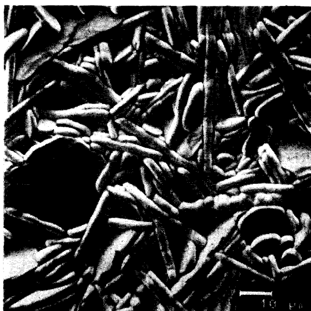
Fig. 9. Microstructure of polished and thermally etched BIT samples sintered at (A) 1050°C and (B) 1100°C.
