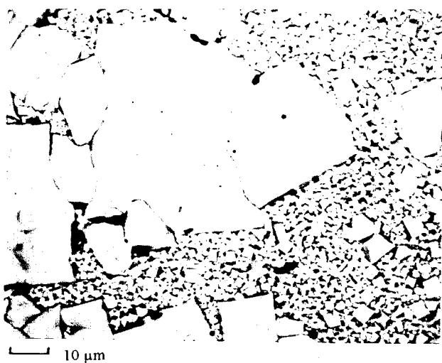
Fig. 2. SEM micrograph of Ti-free \text{In}_2\text{O}_3 ceramics sintered at 1450^\circ\text{C} for 3 h.
