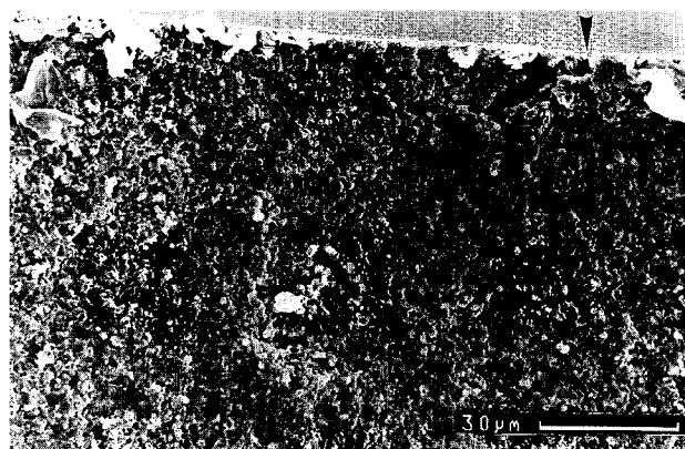
Fig. 5. The presence of surface pore acting as fracture flaw seriously deteriorated the flexural strength of the \alpha -SiC ceramics.
