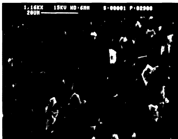
Fig. 4. SEM image showing flake and pellet morphology.
