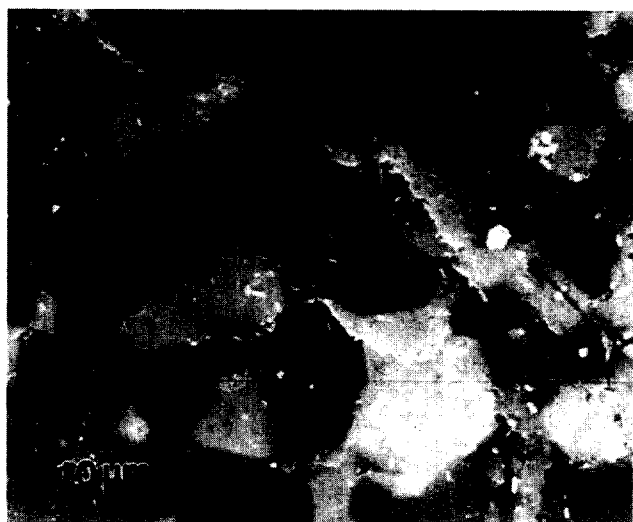
Fig. 11. SEM micrograph showing piled-up wear debris in the recesses caused by differential grain wear rates. The debris in this case was primarily zirconia from the pin.
