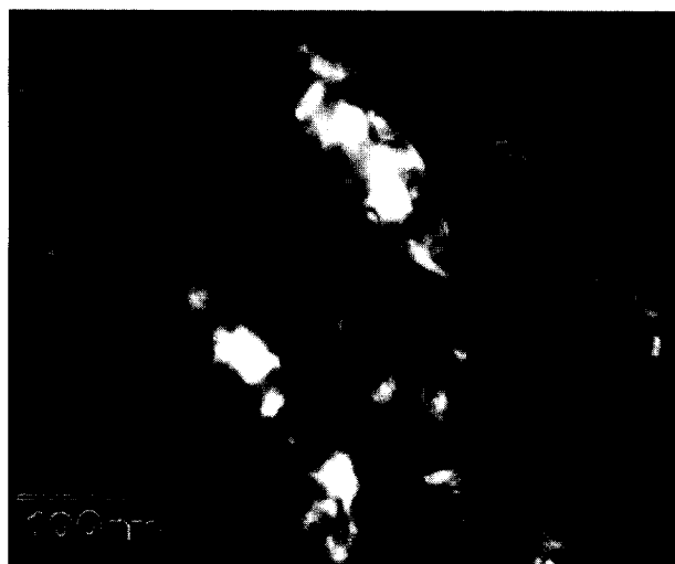
Fig. 5. Dark field TEM micrograph from just below the worn surface of an Mg-PSZ. The majority of the precipitates were tetragonal, with no evidence of plastic deformation. However, the image of the precipitates was clearly distorted by residual elastic strain.
