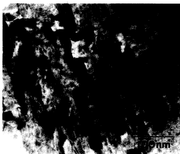
Fig. 6. TEM micrograph from a back-thinned Mg-PSZ showing the structure at the extreme surface. Isolated tetragonal precipitates are present surrounded by an iron based oxide. The cubic appears to have dissolved in the iron oxide. Note the diffuse interface between the zirconia and the transfer layer.
