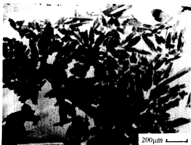
Fig. 2. Transmission electron micrograph of the synthesized hydroxyapatite powder reacted in a pressurized-heating-pot at 109°C for 3 h.
