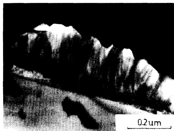
Fig. 3. Microstructure of AlN columnar grains.
