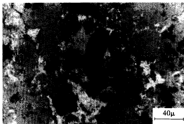
Fig. 5. Optical micrograph of infiltrated sample (AlN + 4% B_4C ).
