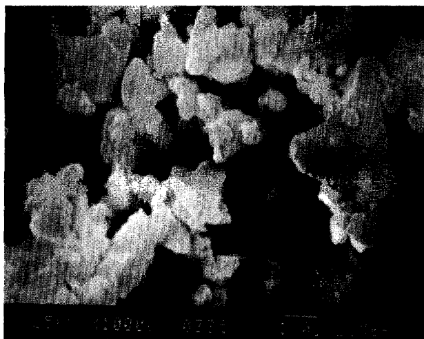
Fig. 1. Scanning electron micrograph (SEM) of unreacted powder: 0.49\text{PbTiO}_3-0.46\text{PbZrO}_3-0.05\text{Pb}(\text{Fe}_{0.2}\text{Ni}_{0.2}\text{Ta}_{0.6})\text{O}_3
