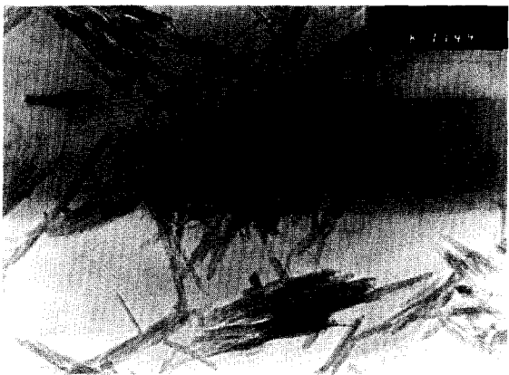
Fig. 5. A TEM photomicrograph of the Sepiolite A sample at room temperature, loose form x16,000.
