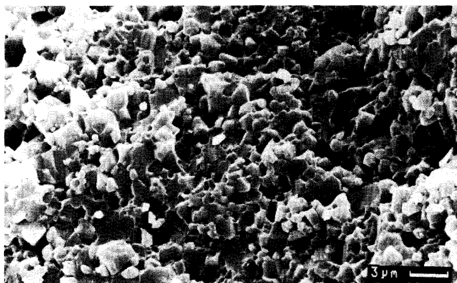
Fig. 1. Scanning electron micrograph of the fractured surface of the SiC ceramic.
