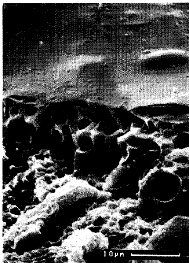
Fig. 11. Spherical pores distributed randomly in the oxide scale formed by oxidation of the SiC with 5 wt% additives at 1350 °C for 30 h.
