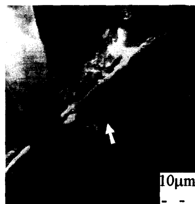
Fig. 11. SEM examinations of the wear debris (dry, 117.6 N, 1.6 m/s).
