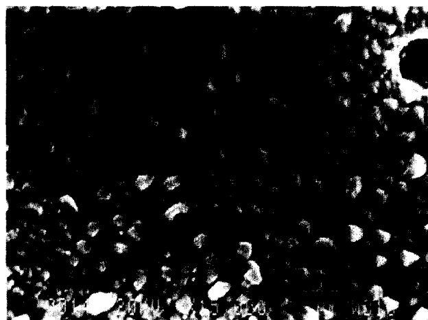
Fig. 5. SEM micrograph of the implanted alumina ( 10^{17} \text{Cr}^+ / \text{cm}^2 , 110 keV) after thermal annealing in air at 1200°C.
