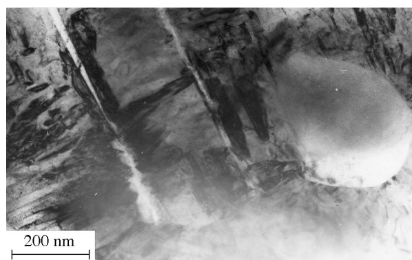
Fig. 4. Typical microstructure including c-, t- and m-ZrO 2 , MgO pipes and MgAl 2 O 4 particles.
