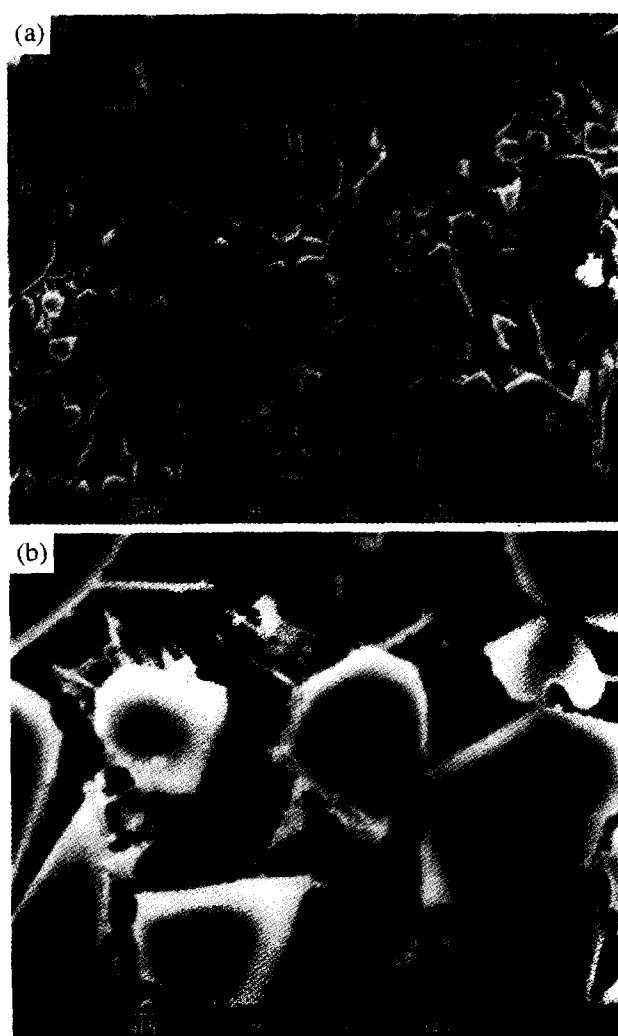
Fig. 3. Secondary electron image of A_{20} composition fired at 1450°C showing: (a) dissolution of sillimanite grains and (b) presence of fine mullite needles in the interstitial spaces.
