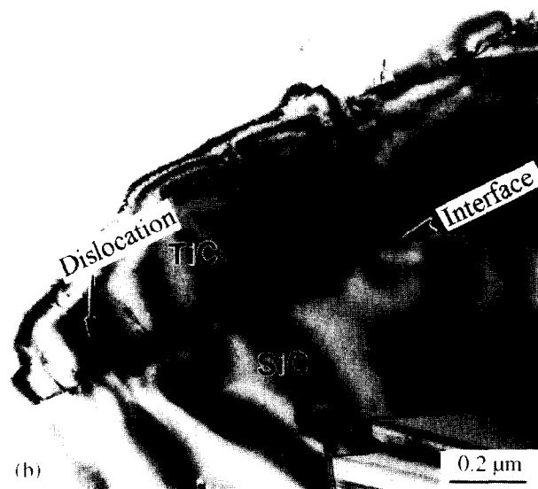
Fig. 10. Microstructure of the SiC-TiC composite observed by TEM for (a) bright field image; (b) SiC-TiC interface micrograph.
