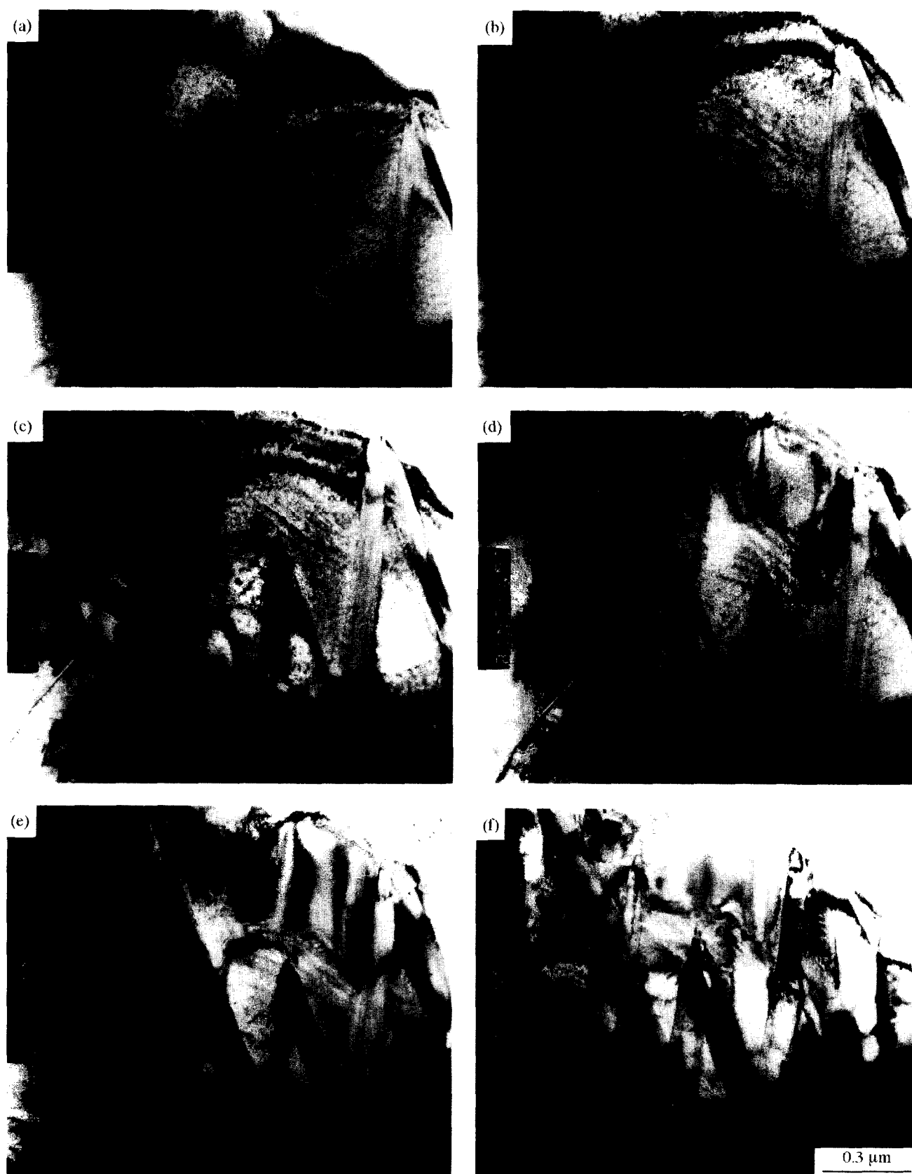
Fig. 1. A series of TEM photographs showing the dynamic process of nucleation and growth of m-ZrO 2 martensite in ZrO 2 -2 mol%Y 2 O 3 ceramics: (a) 20 s; (b) 60 s; (c) 90 s; (d) 150 s; (e) 5 min; (f) 10 min.
