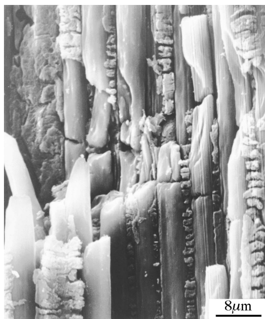
Fig. 12. Orientation of lamellar pitch carbon within fibre bundle.
