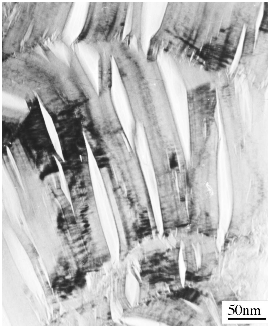
Fig. 10. Orientation of cross-linked lamellar pitch carbon between single filaments.
