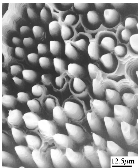
Fig. 6. Z-direction bundles preferentially ablated along the interface. The lamellar CVD carbon was preferentially ablated.
