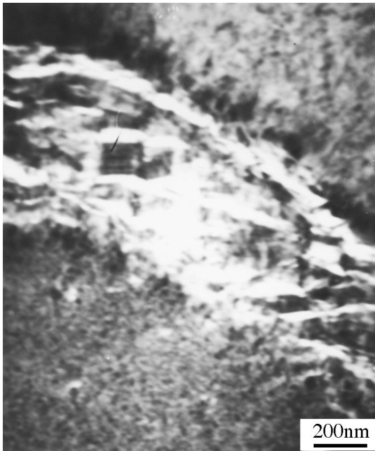
Fig. 3. Lamellar CVD carbon between the dense CVD carbon and the fibre surface.
